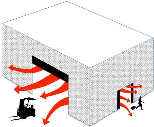
To evaluate the infiltration losses, calculation is made considering heater and cooling operation when inside temperature changes due the massive air exchange during door opening cycles.
