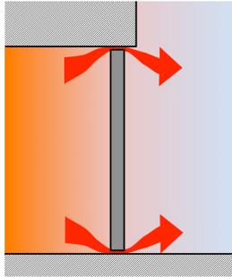
Example Closed Door Leakage Air Flow
