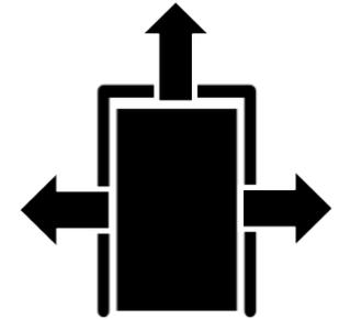
There is a **air flow** that passes through the interstices of the door when it is closed that implies an exchange of heat. The pressure difference between inside and outside can be generated by two factors:
