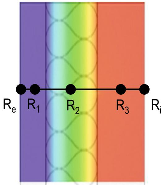
$$U = \frac{1}{\frac{1}{R_e} + \frac{1}{R_1} + \frac{1}{R_2} + \frac{1}{R_3} + \frac{1}{R_i}}$$
